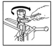
Thread nipple clockwise into socket and hose. Leave 1/32" to 1/16" clearance between nipple hex and socket.
