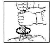
Put socket in vise and rotate hose counterclockwise into socket until it bottoms, then back off 1/4 turn. When assembling long lengths of hose put the hose in vise just tight enough to prevent turning and turn socket into the hose counterclockwise until it bottoms.
