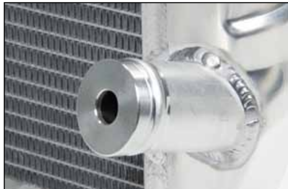
Restrictor Shown Installed Into 1-3/4" Lower Outlet
