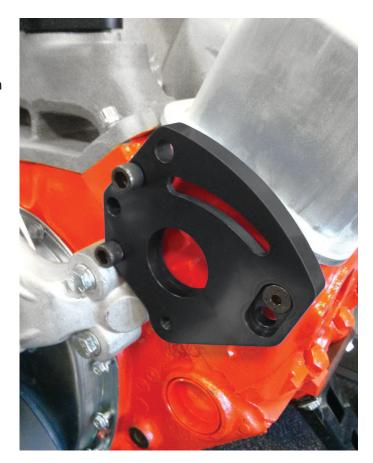
**8.** Rotate pump assembly until proper belt tension is reached and tighten the pump to bracket retainer bolts.
