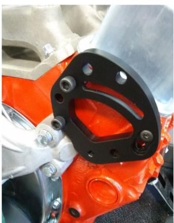
**7.** Rotate pump assembly until proper belt tension is reached and tighten the pump to bracket retainer bolts.
