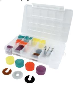
**Bump Stop Pucks** - pucks are replacement components found in ALL64320 Bump Stop Kit in addition to other durometer ratings for even more adjustability. 2.10" O.D. pucks have a 5/8" I.D. hole suitable for 16mm shocks as well as many other uses including suspension limiters.
